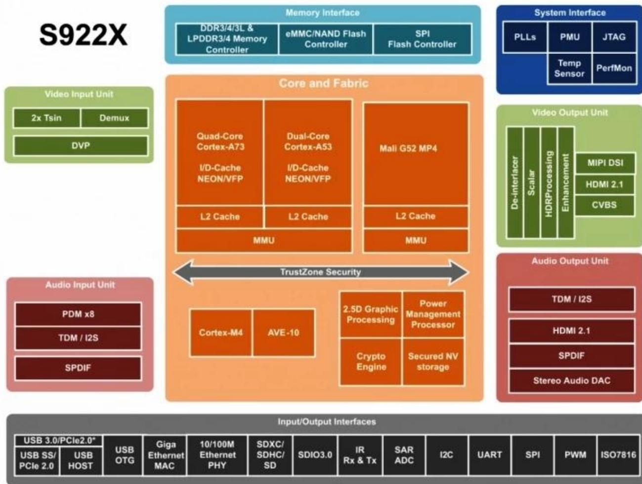
Supported configuration: PCIe2.0 port + USB2.0 Host, or USB3.0 without PCIe
