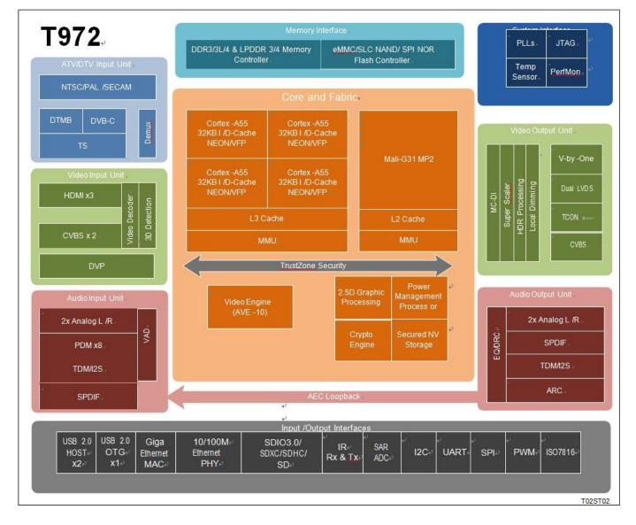
**Amlogic T972** is an advanced application processor designed for worldwide UHD TV applications. It integrates a powerful CPU/GPU subsystem, a best-in-class HDR image processing pipeline, a secured 8K/4K video CODEC engine with all major peripherals to form the ultimate cost-effective smart TV chip.
