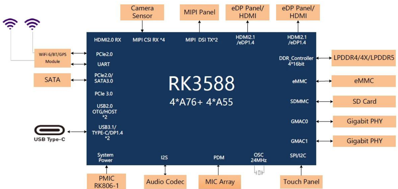
Typical Application Diagram – AIoT
