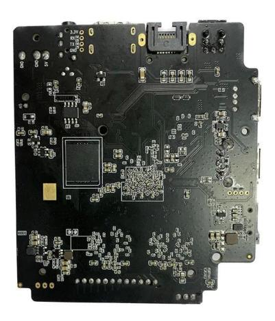
Amlogic S928X is the first 8K UHD smart STB SoC integrating ARM Cortex-A76, ARM Cortex-A55 and self-developed neural network processor. It supports 8Kp60 video decoding function of global mainstream video formats——AV1, H.265, VP9, AVS3, AVS2, etc. Meanwhile, 4K GUI, intelligent SR and other functions are viable as well, thus providing an outstanding hardware engine for customized high-end applications.
