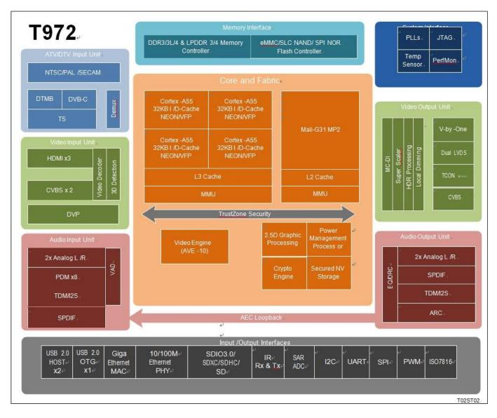
**Amlogic T972** is an advanced application processor designed for worldwide UHD TV applications. It integrates a powerful CPU/GPU subsystem, a best-in-class HDR image processing pipeline, a secured 8K/4K video CODEC engine with all major peripherals to form the ultimate cost-effective smart TV chip.
