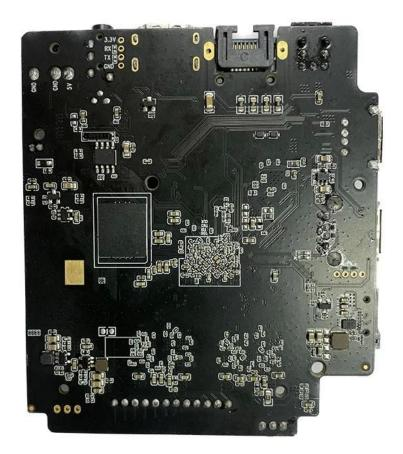
Amlogic S928X-J is the first 8K UHD smart STB SoC integrating ARM Cortex-A76, ARM Cortex-A55 and self-developed neural network processor. It supports 8Kp60 video decoding function of global mainstream video formats——AV1, H.265, VP9, AVS3, AVS2, etc. Meanwhile, 4K GUI, intelligent SR and other functions are viable as well, thus providing an outstanding hardware engine for customized high-end applications.
